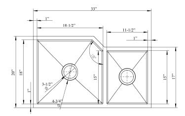
Dimensions of fixture are nominal and may vary within the range of tolerances established by ANSI Standard A112.19.2. Dimensions and specifications subject to change without notice.
